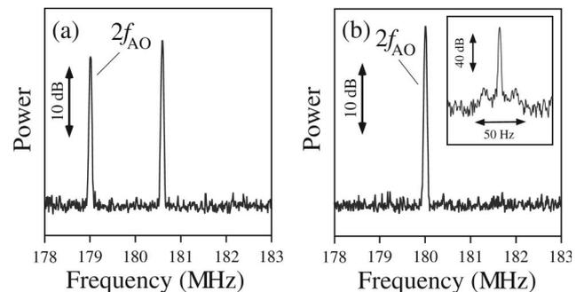
Fig. 3. Typical experimental spectral analysis of the output pulse train power. Resolution bandwidth (RBW) = 30 kHz. (a) Unlocked beat note, i.e.,  $\Delta\nu > \gamma_e/2\pi$ . (b) Locked beat note, i.e.,  $\Delta\nu < \gamma_e/2\pi$ . Inset, RBW = 1 Hz.
