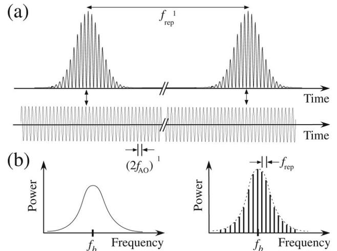
Fig. 2. (a) Schematic of a pulse train (repetition rate  $f_{\text{rep}}$ ) carrying a beat note locked to  $2f_{\text{AO}}$ . (b) Schematic of the output RF spectra corresponding to (left) an incoherent beat note at  $f_b$  delivered by a free-running laser, or to (right) a fully coherent beat note locked to  $f_b = 2f_{\text{AO}}$ .
