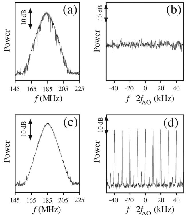
Fig. 6. Experimental spectral analysis of the output power for two different frequency spans.  $f_{\text{AO}} = 92.5 \text{ MHz}$ . (a), (b) Unlocked regime. (c), (d) Locked regime. (a), (c) RBW = 1 MHz. (b), (d) RBW = 300 Hz.
