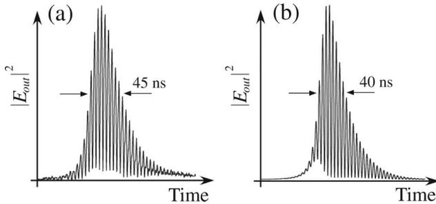
Fig. 5. Output pulse intensity evolution versus time when  $f_{\text{rep}} = 10 \text{ kHz}$  and  $\Delta\nu = 0$ . (a) Experimental pulse. (b) Calculated pulse with the parameters  $g = 0.3$ ,  $R_3 = 0.4$ , and  $\eta = 3$ .
