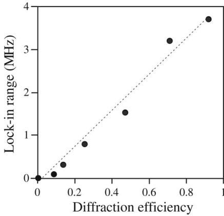
Fig. 4. Experimental cw locking range as a function of the diffraction efficiency of the AO.
