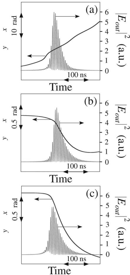
Fig. 7. Calculated intensity and phase difference time evolution for three detunings. (a)  $\Delta\nu = 10$  MHz. (b)  $\Delta\nu = 1$  MHz. (c)  $\Delta\nu = 100$  kHz. The parameters are  $g = 1$ ,  $R_3 = 0.1$ ,  $\eta = 3$ , leading to  $\gamma_e/2\pi = 2.2$  MHz.
